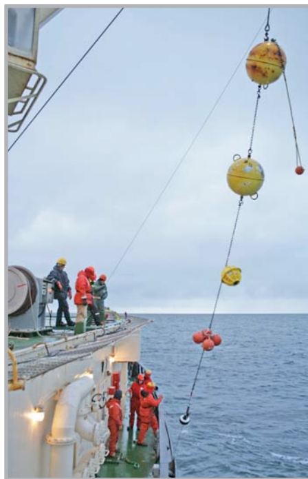
Recovering a deep sea mooring system that had been recording changes in temperature, conductivity, and other characteristics of Arctic Ocean waters. (Source: NOAA At The Ends of the Earth Collection)
